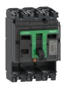
Circuit breaker basic frame, ComPacT NSX100H, 70kA at 415VAC 50/60 Hz, 100A, without trip unit, 3 poles
