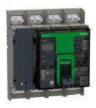
Circuit breaker, ComPacT NS1250N, 50kA at 415VAC, 4P, fixed, manually operated, MicroLogic 2.0A control unit, 1250A
