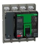
Circuit breaker, ComPacT NS1250N, 50kA at 415VAC, 4P, fixed, manually operated, MicroLogic 5.0E control unit, 1250A
