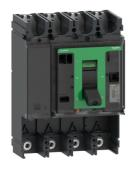
Circuit breaker basic frame, ComPacT NSX400F, 36kA at 415VAC 50/60 Hz, 400A, without trip unit, 4 poles
