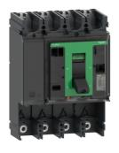
Circuit breaker basic frame, ComPacT NSX630H, 70kA at 415VAC 50/60 Hz, 630A, without trip unit, 4 poles
